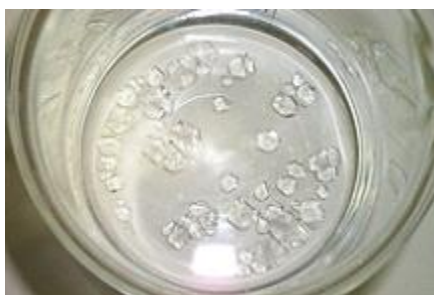
Figure 2. Seed crystals of alum. (Credit: picture by Luc Van Meervelt)
