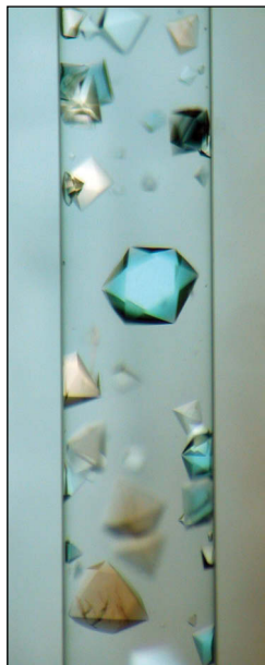
LEC: Crystallization under diffusion-controlled mass transport.
