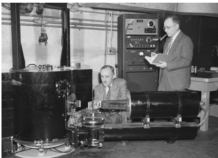
Clifford Shull (right) and Ernest O. Wollan with a neutron double crystal spectrometer at the ORNL X-10 graphite reactor, in 1949.
